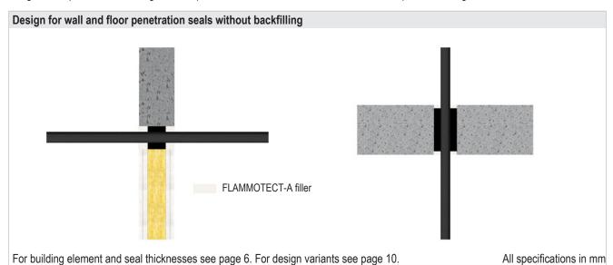
Service  $\begin{array}{c|cccc} \textbf{Diameter} & \textbf{FLAMMOTECT-A filler} & \textbf{Fire resistance class} \\ \hline \textbf{Dry film thickness [mm]} & \textbf{Wall} & \textbf{Floor} \\ \hline \textbf{Cables} & & \geq 25 & \textbf{EI 90} & \textbf{EI 90} \\ \hline & \geq 3 & - & \textbf{EI 90} \\ \hline \end{array}$
